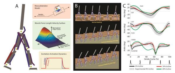
**Figure 1**: (A) Musculoskeletal model; (B) Simulated predictions of the gait cycle of normal walking and inclined walking at 10 and 20 degree inclines; (C) Sagittal hip, knee, and ankle gait kinematics of normal walking and inclined walking at 10 and 20 degree inclines.
